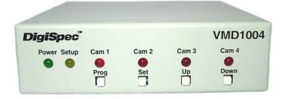
The VM D1004 is a 4 camera video switcher that has VMD (Video Motion Detection) on each camera. OSD (On-Screen) programming for switching dwell time, bypassing and motion dwell time along with the VMD setups is all done via 4 front panel pushbuttons. Independent defined motion areas and sensitivity for each camera. One video output will be able to drive two 75 ohm video loads at 1VP-P. One hard alarm output is provided whenever any camera goes into motion alarm mode.
